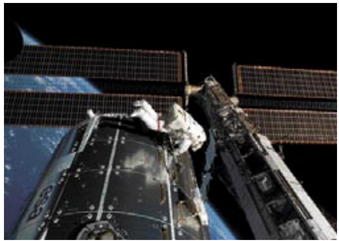
A panoramic view of a mission specialist US astronaut installing handrails on the outside of the International Space Station in 2008
